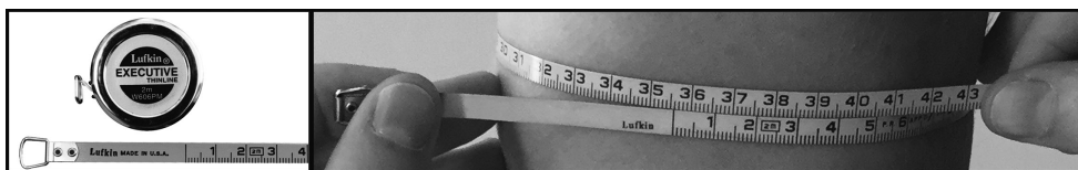
Figure 4.2 Anthropometry tapes are shown on the left. The right image shows how to read the tape where the zero mark is aligned with the top scale: here reading 35.6 cm
